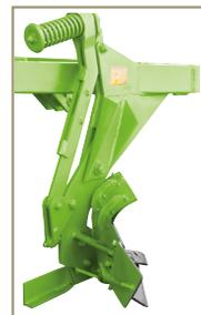
Equipped with Special Shock Control that disarm when the Mouldboard finds an obstacle and rearm automatically with simples lifting of the implement.
