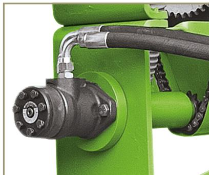
Operation of the fertilizer dosing valve through the hydraulic motor.
