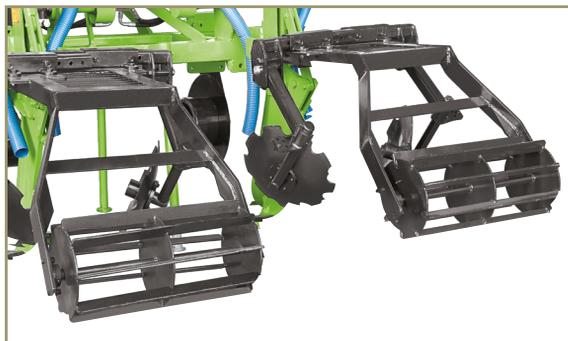
Set of trimmed disks and leveling rolls.
